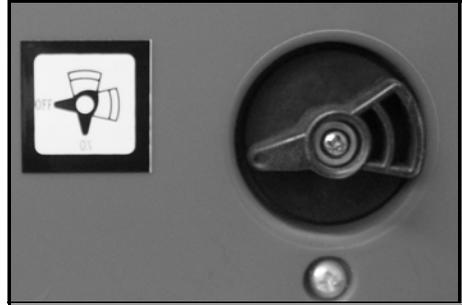
3. Turn the air vent knob to the off position.
