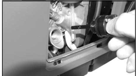
5. If the oil is below the Min. level on the dipstick, add oil to the oil reservoir.
