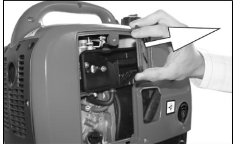
4. Remove the air filter element.
