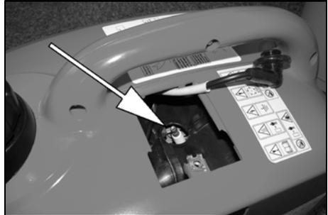
5. Check the spark plug gap (a), it should be between 0.6 and 0.7 mm, adjust if necessary.
