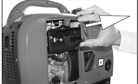
4. Remove the air filter element.
